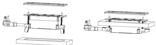
\*Thickness of the board:8~35mm
