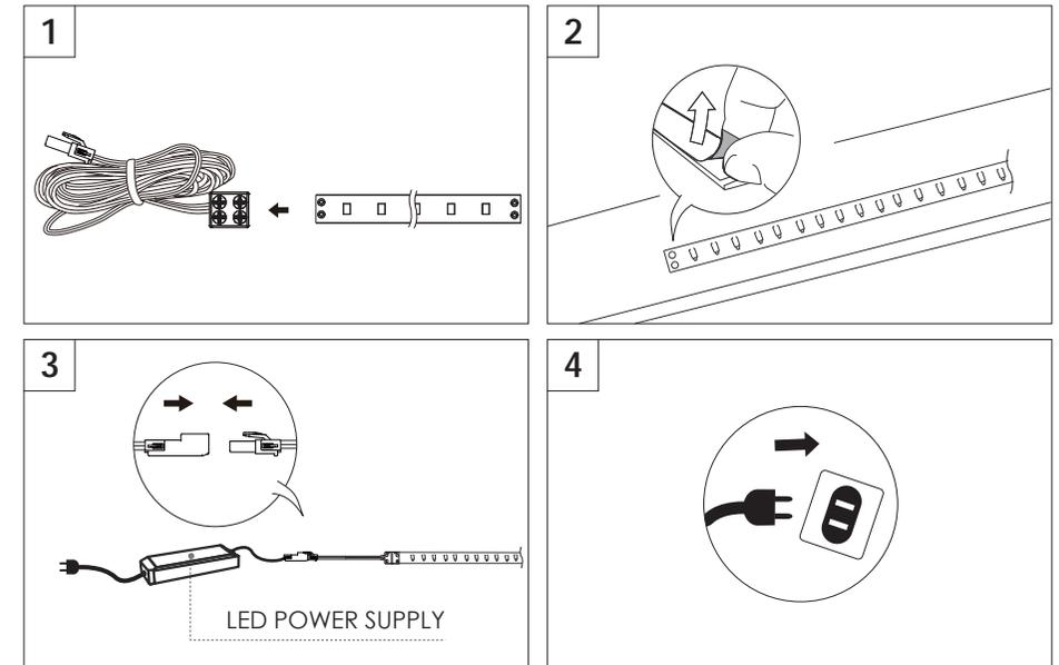
**i** Install LED fixtures with mounting channel:
