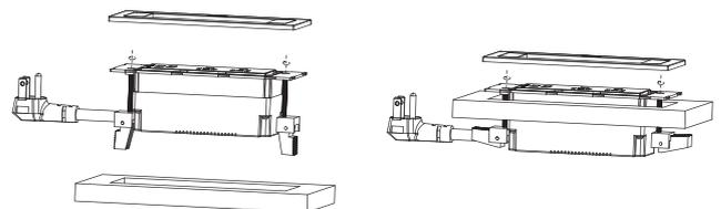
\*Thickness of the board:8~35mm
