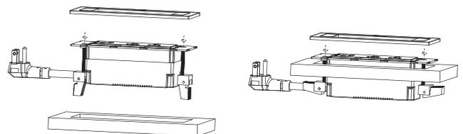
\*Thickness of the board:8~35mm
