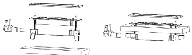
\*Thickness of the board:8~35mm
