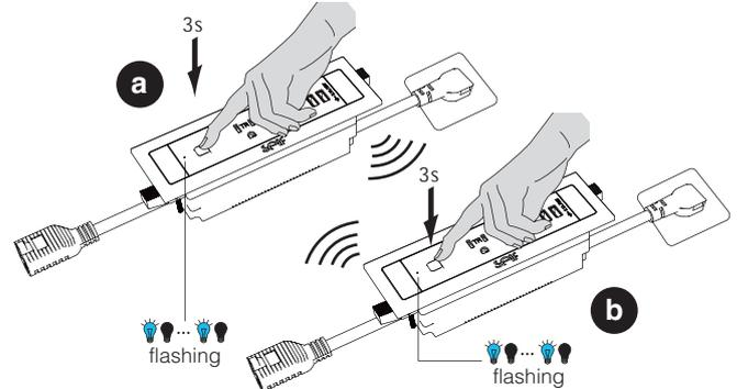
**4** press any paired power unit's switch, all the lights that powered by paired power units can be controlled.
