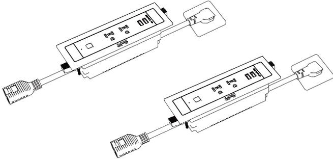
**3** Short press the button of any power unit, the blue indicator will stop flashing and stay ON or OFF, means the pairing is successful.
